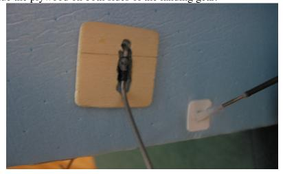
Cut two strips of plywood or plastic that will insert in front and back of landing gear slit.
