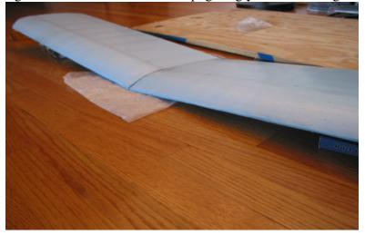
Mix up 5 min. epoxy and glue the wings together. Pour extra into wide seam to fill space. Don't worry about filling the gap completely, we'll do that later with the Hot Glue gun. After top dries, turn over and add 5 min. epoxy to seam again.
