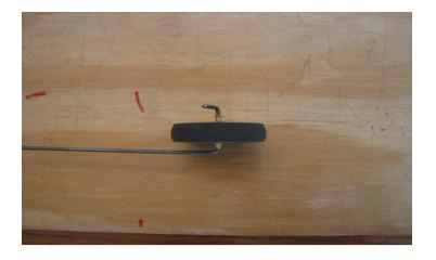
Poke two skewers into fuse on both sides of wire for support and Epoxy.
