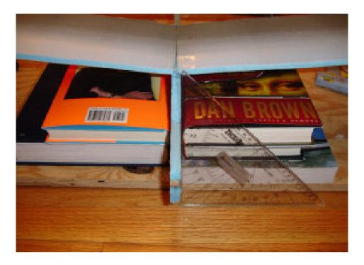
Place fuse between books and make sure it's straight. Prop wings up with books at the wing tips and measure. Make sure they are equal height and they match the leading and trailing line marks on the plans.
