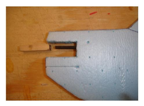
Add a small amount of 5 min epoxy and slide over CF rod.
