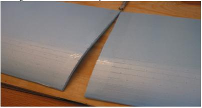
Lay down a piece of waxpaper to protect the table surface and place the wing seam on it.
