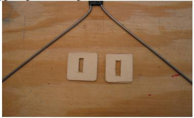
Cut a slit in the fuselage 5 3/4 inches back from the nose and 1/2 inche from the bottom of the fuse. Insert gear.
