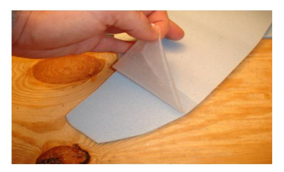
Separate the two fuselage pieces and peel the skin off the inside (not outside) halves that will be glued together.
