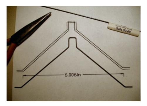
Using the template from the plans and .055 music wire, bend the landing gear into shape.  $\,$
