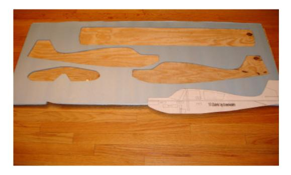
Trace along the outside edge and remove plans. Using a sharp, new #11 exacto knife, cut out the STC, holding the knife straight. Take your time and make smooth long cuts
