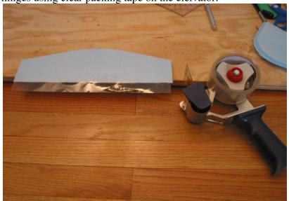
Deflect elevator 45 degrees before pressing tape down.
