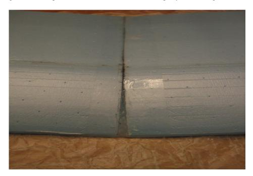
After epoxy dries, fill any gaps with Hot glue. Wrap seam in clear packing tape.
