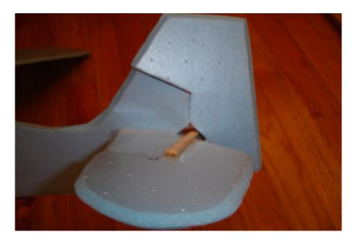
Now attach rudder using packing tape, same as before with elevator. Cut hole for reinforcement wood stick to move freely up and down.
