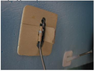
Align gear. Pour 5 min.epoxy or hot glue into slit. Allow to dry.
