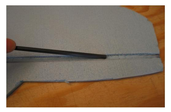
Cut a shallow groove along the line on both inside halves using a rod.. (The cutout template of the fuselage has a line running from nose to tail, use that as a guide) Using the end of the 1/8in.carbon fiber rod (recommended) or dowel, press down on the foam as you drag it down the groove, to make the cut.
