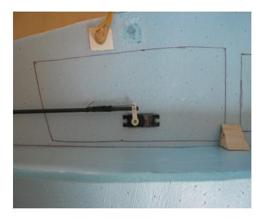
Using the .032 music wire, bend control rods. Before bending both ends, slide coffee straws or WD40 tubes over them. Hot glue them to the fuse to support the wire.
