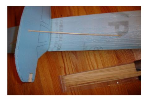
Using 12 in or longer bamboo skewers, hot glue the struts in to place.
