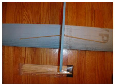
On opposite side in fuselage, poke the bottom of the strut through the foam until it butts up against the bottom of the other strut. Hot glue them together in fuse and attach other end to wing.
