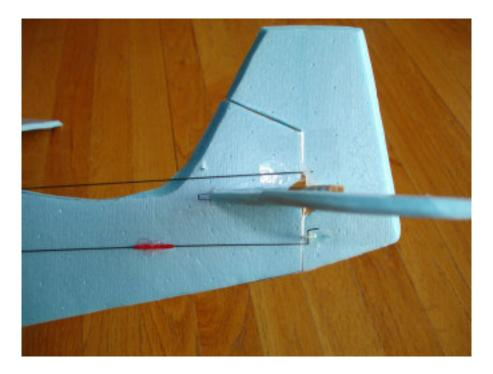
Add a ESC, 3-4 channel receiver, and motor. Use Velcro for easy removal. This is a 20mm CDROM motor rewound with 18 turns of 26g. wire and N50 magnets and a 8040 DD prop. Or use the single or double ISP-A motor with a 9 in. prop.
