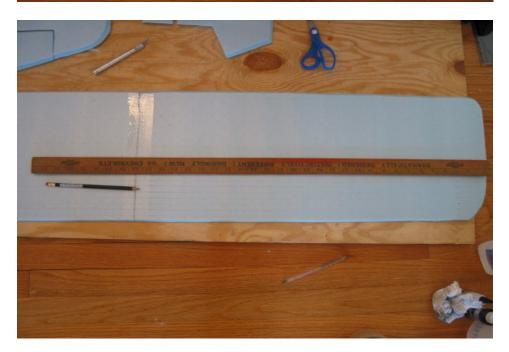
Don't press down too hard with the pencil, just enough to leave a visible line. Depron is more brittle than blucor. To prevent breakage, wrap clear packing tape along the leading edge, wing tip to wing tip, before next step.
