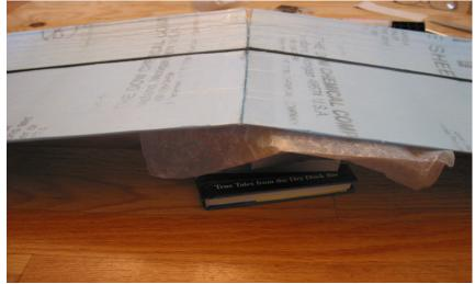
Run clear packing tape down the leading edge and down the spar, top and bottom.
