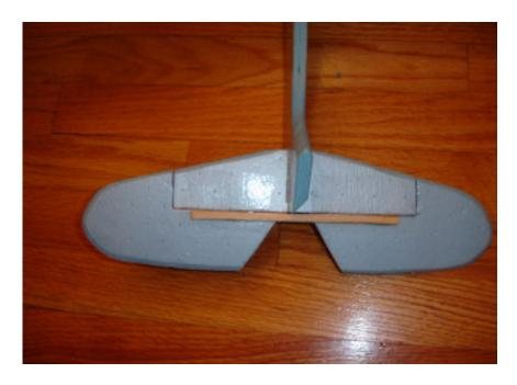
Now attach the "tailfeathers" to the fuse using 5 min. epoxy. Be sure they are straight and true. Measure front wing tip to rear wing tip. If both sides are even, your straight.
