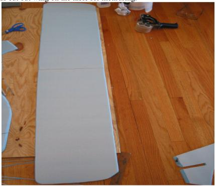
Using a ruler and a pencil, draw lines along the leading edge of the wing, spacing them a
