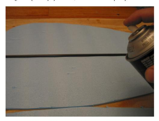
Light to medium coverage will hold fine. Heavier along carbon fiber groove.
