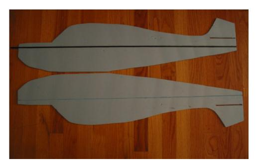
Place the carbon fiber rod (or dowel) in the groove and press both halves together.
