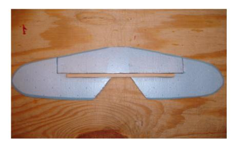
Using a 1/8 x ½ in. basswood as reinforcement for the elevator. Epoxy into place.
