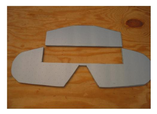
Place the fuse aside to dry, grab the stab/elevator pieces and finish cutting them out.
