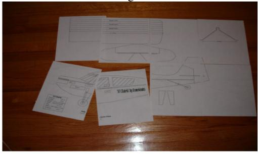
Tape tiled plans together to make full size plan. With full size or tiled plans that have been taped, cut out the STC and tape to the foam.
