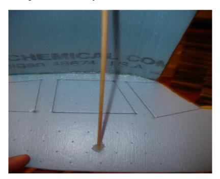
Lift wing off and add 5 min epoxy (or hot glue for easy removal later if you decide to change wing incidence) to the wing saddle. Place wing back on fuse and measure tips. Don't worry about any gaps, we'll fill them with hot glue after the wing dries.
